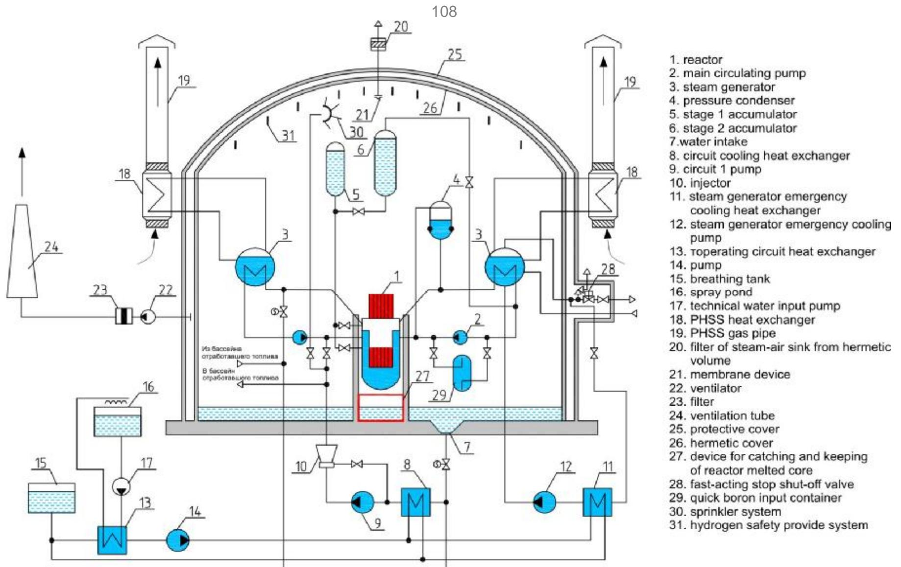
Figure 26 – Energy unit safety system diagram
