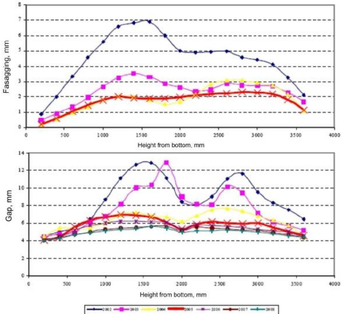
**Figure 15 – Changing of bends and inter cassettes clearances in plant 1 at increasing FA-2 in the area**
