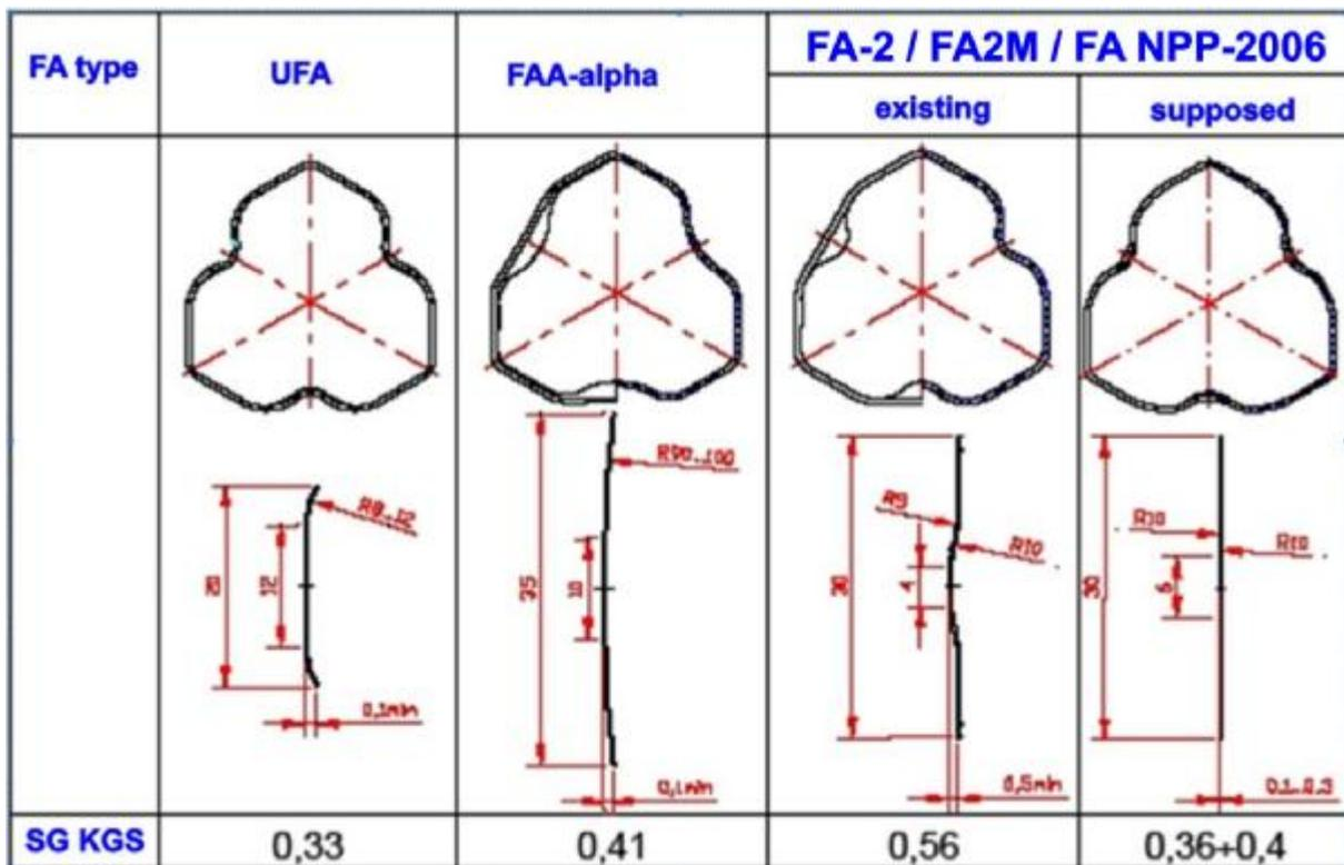
**Figure 12 – SH cells of different FA types**
