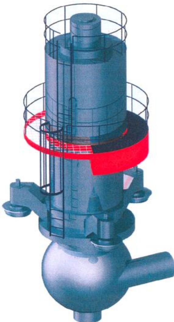
**Figure 24 – Main circulating aggregate**
