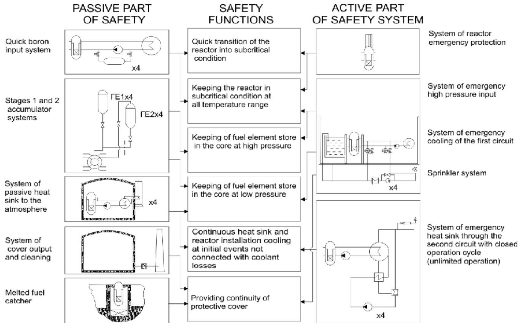
Figure 27 – Basic solutions on providing safety functions in project NPP-92
