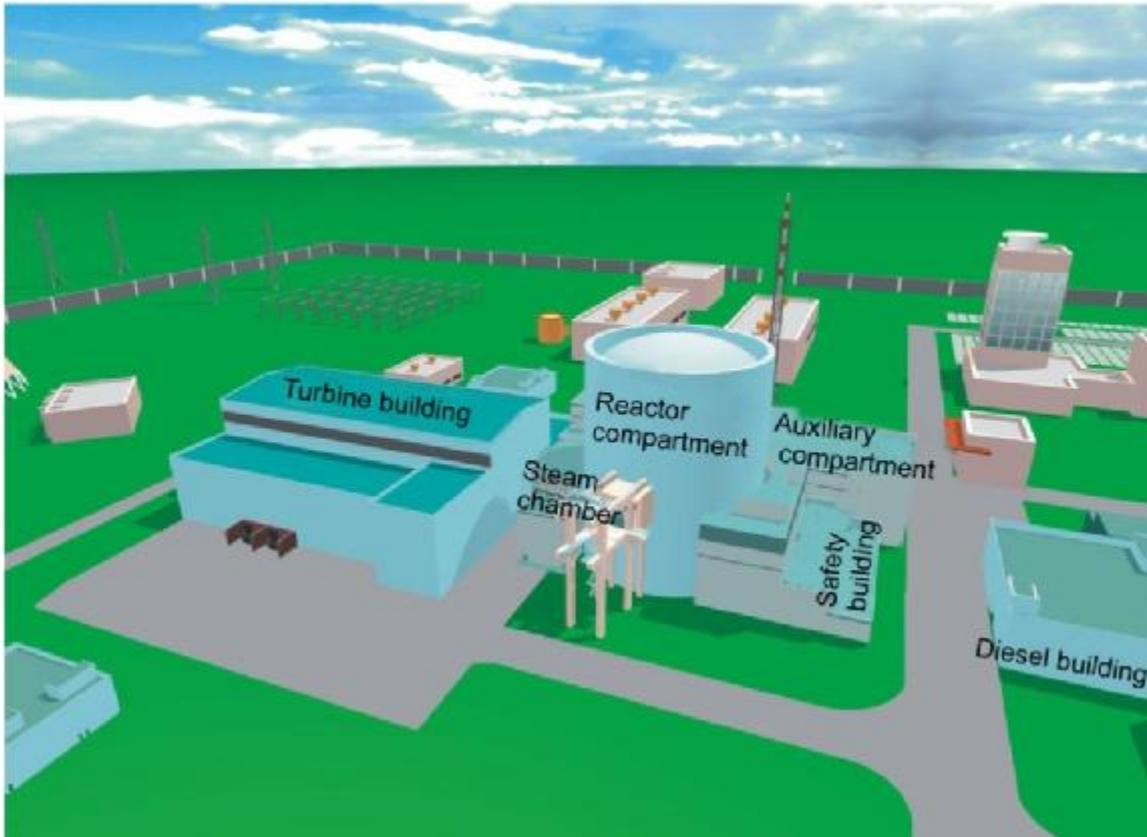
**Figure 6 – Overall view of one-unit NPP**
