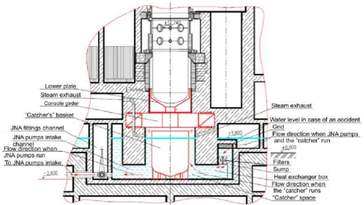
**Figure 28 - Core “catcher” components**
