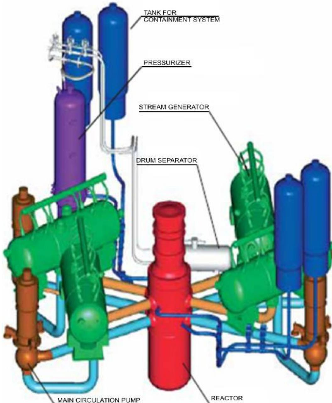
**Figure 7 - Arrangement of reactor installation is shown**
