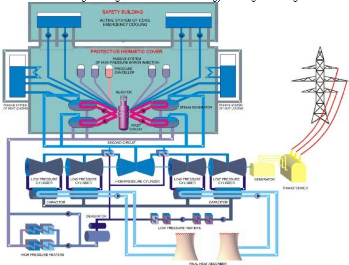
Figure 8 – Functional technological diagram
