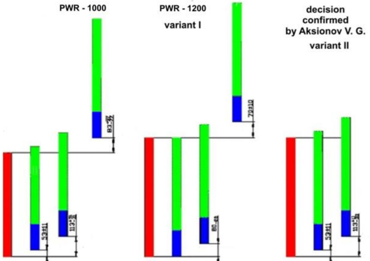
**Figure 18 – Relative positions of fuel and absorber**
