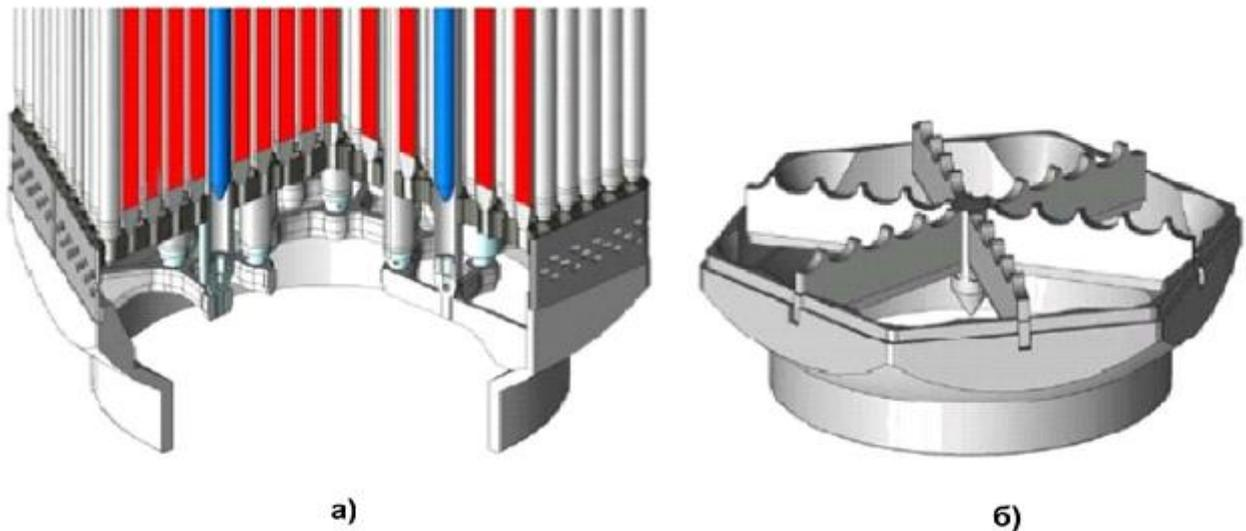
**Figure 17 – Shank end with long NK a) and standard FA-2M shaft end b)**
